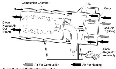
Figure 2 - Cross Section Operational View
